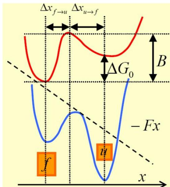
Find out what the change in length of the hairpin construct is as it unfolds. As the measured signals are noisy, this is probably best done by histogramming the time-series, and fitting Gaussians to the peaks in the histogram. Use a time-series where the peaks are well-defined (the molecule spends roughly 50% in each state)
