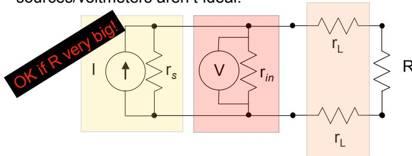
Resistance of the leads means that the resistor looks like
