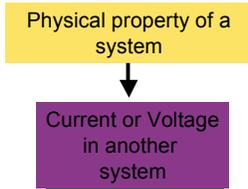
To take advantage of the power of electronics, use a **transducer** - a device which converts a measured physical effect into a signal measured by electronics (normally a voltage or current).
