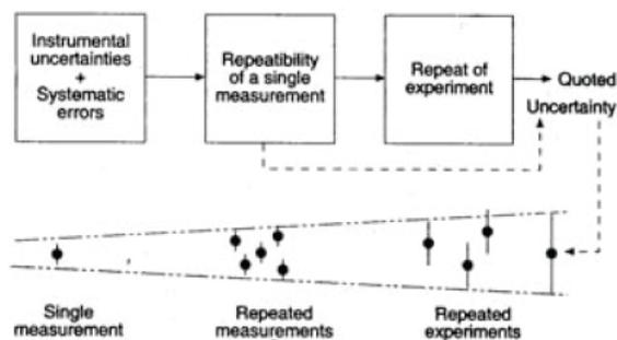
Fig. 1.6 The progression in the uncertainty from that of a single measurement to that for a system.
