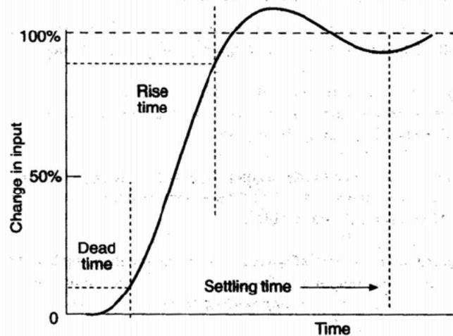
Fig. 2.4 The time response of an instrument after a change in the measured parameter.
